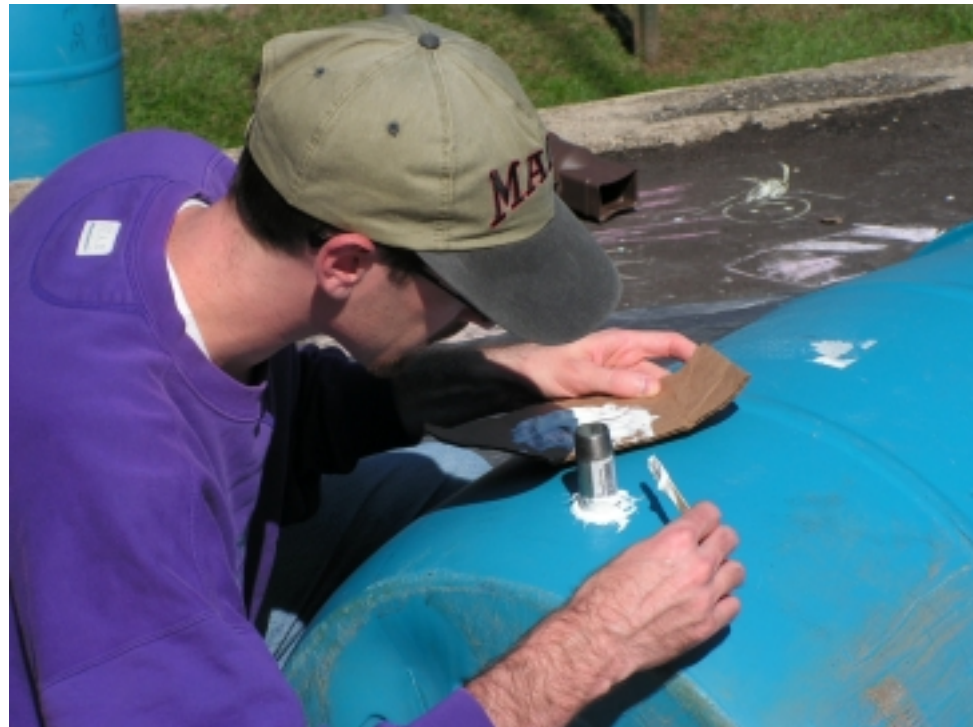
Photo 2. Epoxy sealing lower outlet, after drilling hole.
