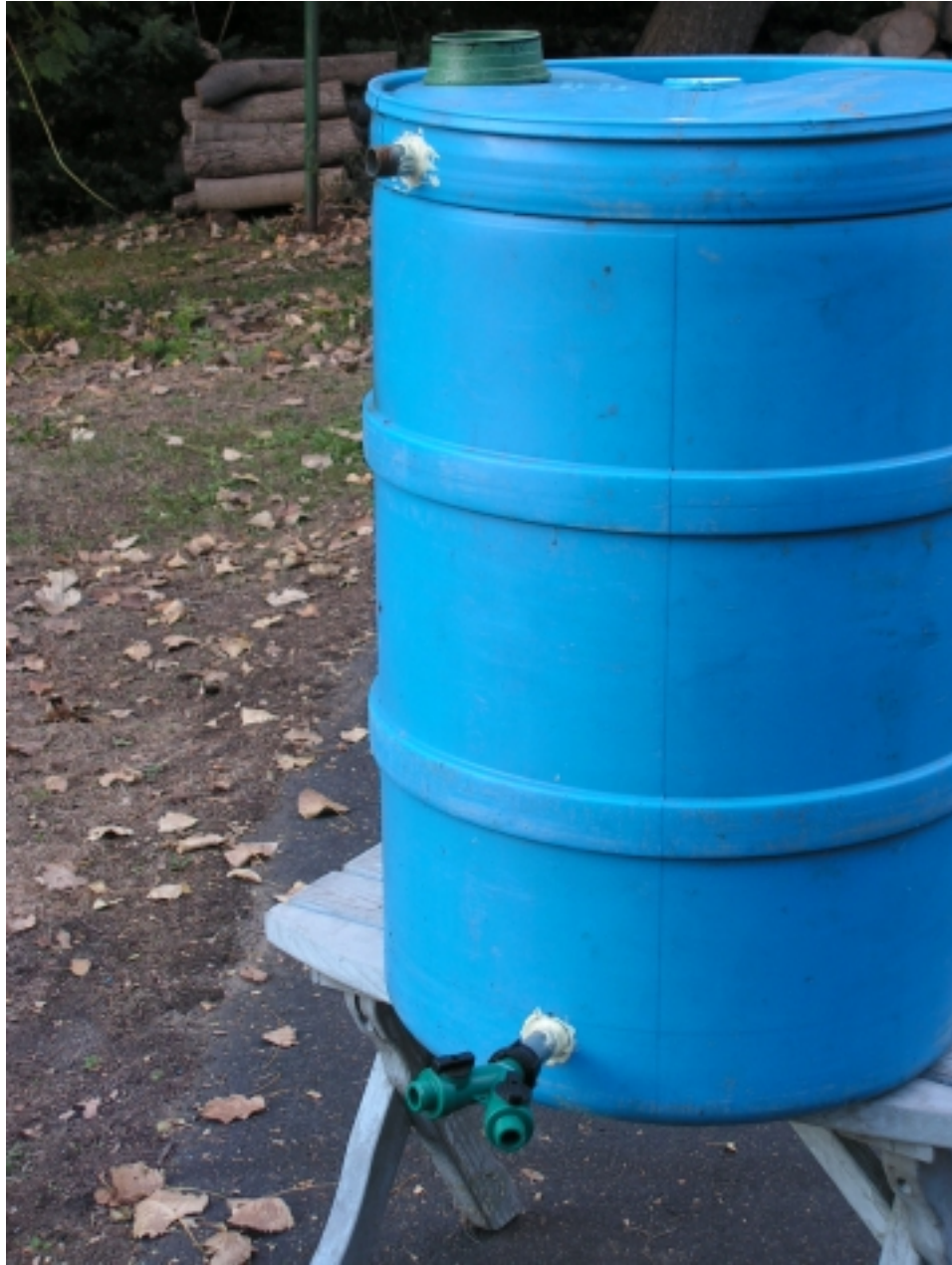
Photo 3. Modified Barrel - Inlet, Overflow, and Outlet
